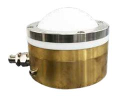
The LOMT Oracle RC is a self-contained, flameproof (Ex d) radio control data transceiver supporting radio remote control of mobile mining machinery. The module communicates with a variety of Pempekmanufactured handheld remote control consoles via a 2-way radio data stream (based on the 915 MHz band).
