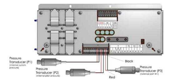
HBox 5  $\mid$  Internal Wiring - CAN ID and Diagnostic Cable
