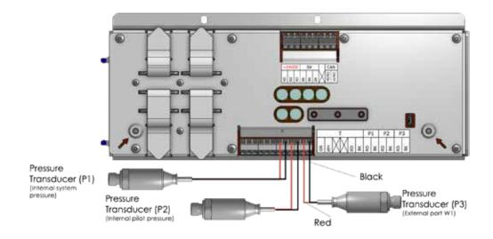
HBox 5 | Internal Wiring - CAN ID and Diagnostic Cable
