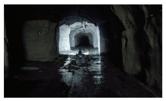
The operator must drive all of the terrain that is to be the operating space of the subject Shuttle robot. The output of the drive through is a point cloud that consists of millions of coordinate vectors.
