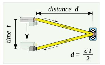
The Pempek Lidar is multi-line laser using time of flight to accurately map the local terrain.
