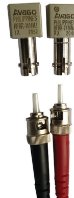
Image above Fibre Optic Patch ST-ST Multi-Mode
