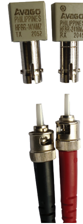
Image above Fibre Optic Patch ST-ST Multi-Mode
